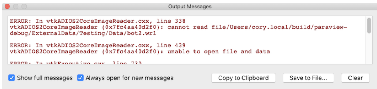
Fig. 1.13: The Output Messages window is used to show errors, warnings, and other messages raised by the application.
